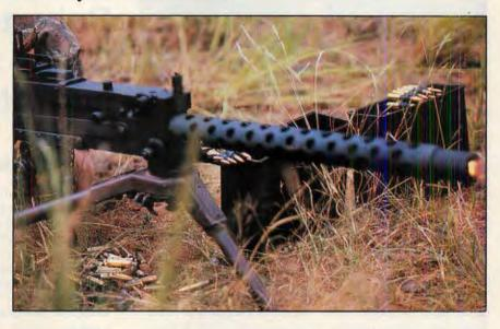
Employed in the light machine gun role of the original M1919A4, the MG4 AA conversion in 7.62x51mm NATO still cranks 'em out with astounding reliability. When converted for use in the co-axial role without sights or pistol grip it is designated the MG4 CA. Canada took a look at what else was available in the 1950s, and converted her M1919A4 Brownings to the C1 in 7.62x51mm NATO, and the U.S. Navy likewise converted a number as the Mark 21 Model O. The South African conversion is simpler.
